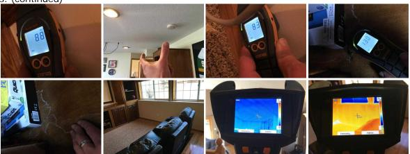
18. All Living Areas Living Space Windows: Vinyl Casement and Sliders - Staining noted on most window frames. These areas tested within acceptable ranges at the time of inspection. May be due to condensation or exterior
